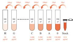
6. Prepare dilutions of the standard as shown in Page 4 and Table 1 below. Vortex each tube and switch each tip between dilutions
